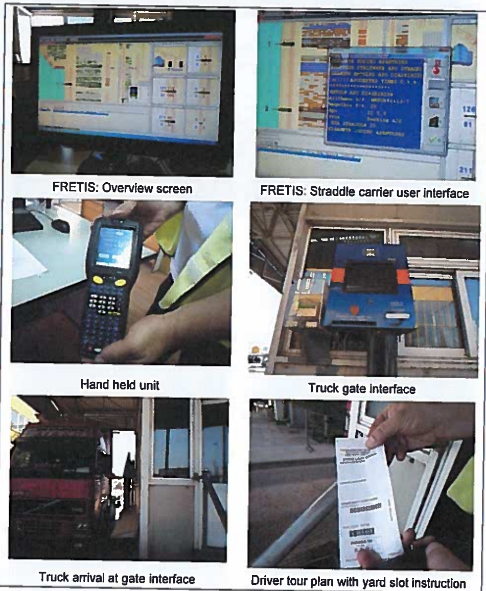
Figure 10: TOS installed at Thessaloniki Container Terminal
